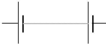
Battery (long terminal is +)
